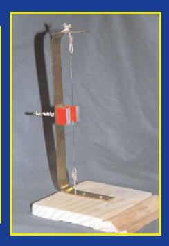
Connect two wire leads from the battery terminals. Alligator clips are helpful for securing the opposite ends of the leads to the flexible wire. (Be sure to strip or sand the insulation from the flexible wire to insure good contacts.) A switch in the circuit can aid in your presentation. Observe the flexible wire move when the current is applied. The movement may be determined by the size, strength and exact shape of the horseshoe magnet.
