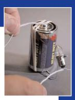
Now try the experiment with a rubber band and string. The bulb will not come on. This is because rubber and cotton fibers are **insulators**. They will not allow electricity to pass, and thus, will not complete the electrical circuit. Now repeat this experiment with other objects. Can you classify these materials as conductors or insulators?
