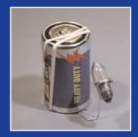
1.) Bend the paper clip at a right angle. 2.) Bend a small loop in one end of the paper clip [Hint: a fat pencil helps] 3. Angle the loop backwards slightly and place the flashlight bulb inside the loop. 4. Double the heavy rubber band and secure the paper clip firmly to the bottom of the battery. [Hint: sanding the paper clip where it touches the battery and bulb helps make good electrical contacts.
